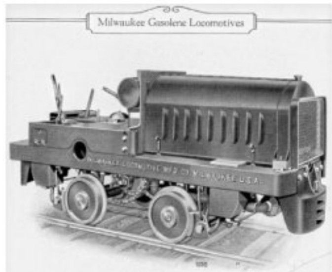
Abandoned remains of a locomotive chassis (above) that operated between camps 2 and 3. The gasoline locomotive corresponds to the W-20 model (below) with 20 horsepower, which was the smallest and most economical model of that time.
