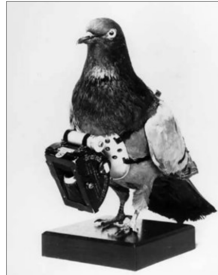
In 1903, Dr. Julius Neubronner patented a miniature pigeon camera activated by a timing mechanism. Equipped with the cameras, the pigeons photographed a castle in Kronberg, Germany around 1908.
