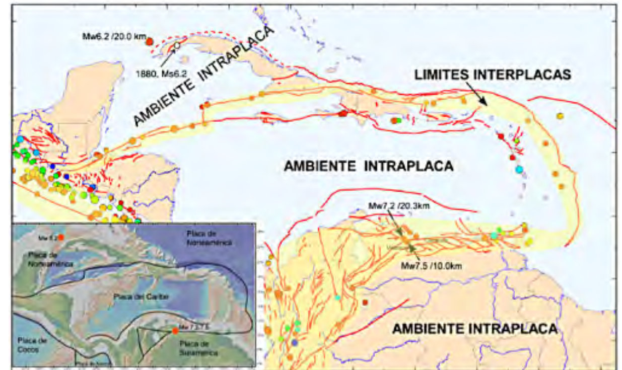
Figure 1. Map of the main faults of the Caribbean and the epicenters of earthquakes of magnitude 6 and greater. Interplate boundaries (yellow) and intraplate zones are highlighted, as well as the position of the epicenters of the June 8 earthquake NW of Cuba and June 24 earthquake N of Venezuela.
