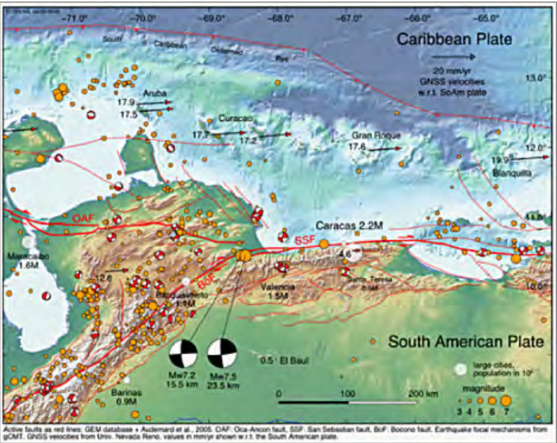
Figure 5. Seismotectonic map of northern Venezuela, including the epicenters of the seismic doublet, courtesy of Eric Calais. Red lines: active faults; OAF Oca-Ancón Fault, SSF San Sebastián Fault, BoF Boconó Fault.
